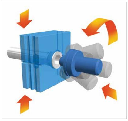
Exclusive Orbital Spindle motion produces a high-quality, reliable flange or flare.
